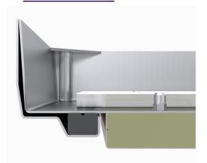
Graphite based intumescent seal, which creates high pressure on expansion. In order to guarantee a secure seal against the spread of smoke and fire, the seal engages at 150°C, ensuring the joints to close quickly to block the spread of smoke and fire.
